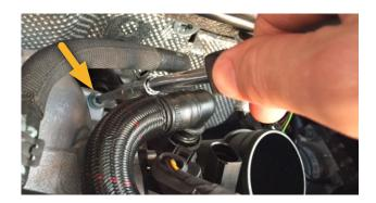
Rotate the top of the intake elbow towards the firewall to disengage it from the turbo as shown below.
