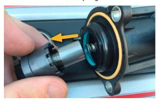
Remove the plastic piston shroud from the solenoid. This should be able to be removed by hand, but if it does need to be levered out take care not to damage any of the plastic pieces.
