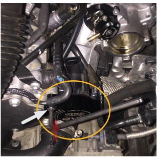
Push the free end of the vacuum hose onto the DVX barb, then clip the wiring connector onto the solenoid.
