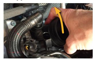
Now unscrew the 3 screws holding the diverter valve (yellow arrows, use a 5mm metric hex key), then remove it from the car. Take care not to drop these screws as they can be difficult to retrieve.
