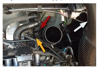
Using a Torx T30 driver, loosen the single screw (yellow arrow above right) that retains the plastic turbo intake elbow.
