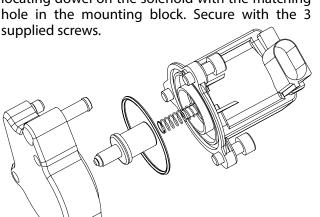
Check that the DVX valve has the two supplied o-rings installed in the grooves, then install it on the turbo compressor cover. The orientation is important - the atmosphere venting port MUST face AWAY from the turbo compressor inlet as shown below by the yellow arrow. Secure with the 3 factory screws.
