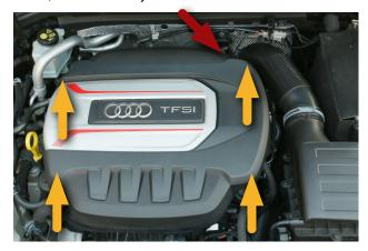
Unclip the PCV hose (red arrow below) and diverter valve electrical connector (yellow arrow), then loosen the hose clamp and remove the intake pipe (white arrow).
