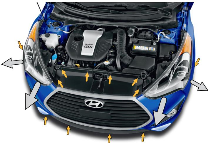
Remove the vacuum hose ( ➔ ) from the factory valve, then unscrew the 3 screws as shown below ( ➔ ).
