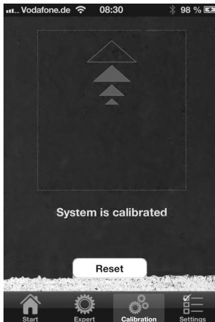
As soon as the calibration is been finished, you get that information on the display of your smartphone. The smartphone can be used normally now and the orientation in driving direction is no longer requested.
