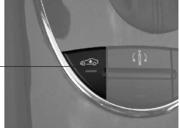
■ Initially lower the lifting platform slowly and only lower completely when the vehicle raises of its own accord.
