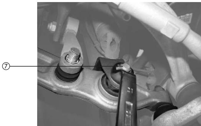
■ Assemble strut fork on the bottom track control arm ⑦.
