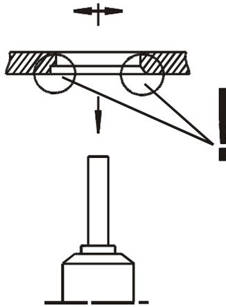
When fitting the spring plate ( 1 ) care must be taken to ensure that the circlip ring ( 2 ) is seated correctly!
