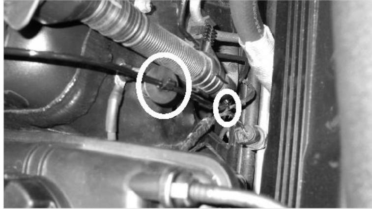
Guide the cable parallel to the filler neck of wipe-and-wash system at passenger's side and attach it with cable strips delivered by BILSTEIN on the threaded pin beneath the ground connection.
