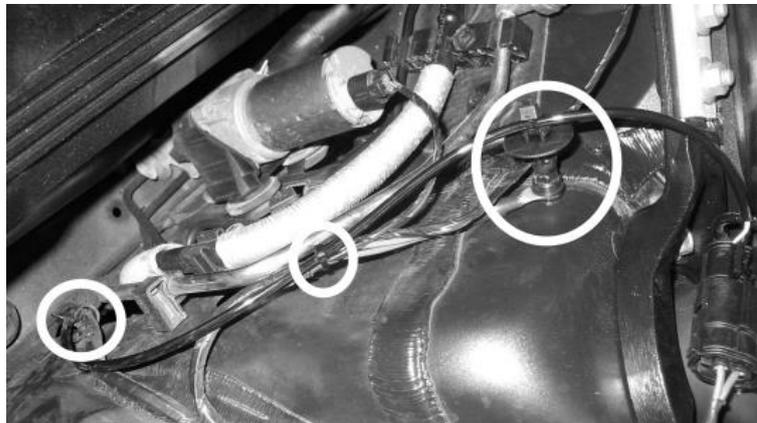
Secure the cable on driver's side to the cable holder of an original cable harness and guide it parallel to the air condition wire. Finally secure it by using a cable strip to the threaded pin of ground terminal. Before the installation of the front cable harness it might be helpful to remove the air-cleaner box.
