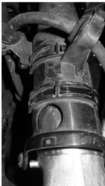
Fixing of original brake hose holder (plastic) by using both cable strips delivered by BILSTEIN, same as original.
