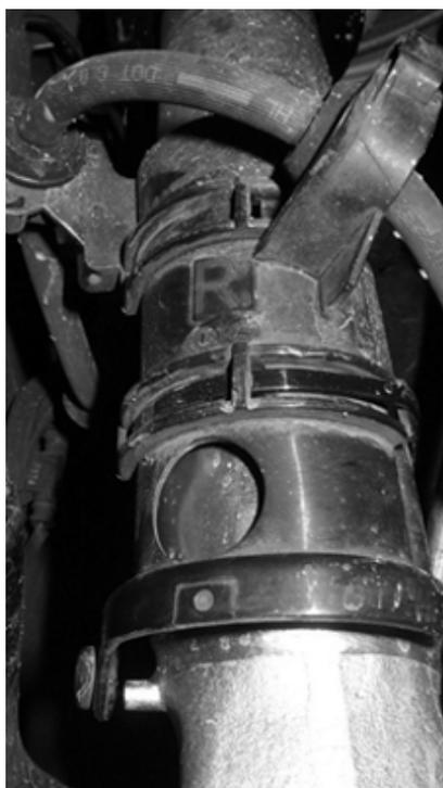
Fixing of original brake hose holder (plastic) by using both cable strips delivered by BILSTEIN, same as original.
