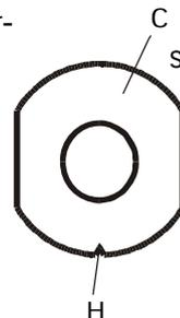
Orient the score mark ( H ) on adjusting head in the centre of any of the four sides of the square rod stop. Then lock the parts together by screwing the lock nut up to the adjuster head.
