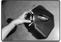
**10.** Rotate the twist lock filter in either direction a 1/4" turn untill the filter locks.
