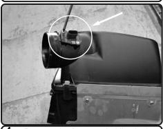
**4.** Remove the 2 screws holding in the MAF sensor using T25 torx bit.
