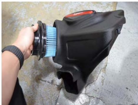
11. Install the twist lock filter on to the Injen air box. Once seated, rotate the filter a 1/4 turn in either direction so the filter can lock into place.
