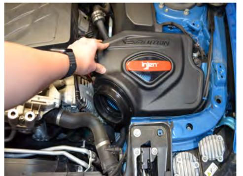
12. Install the Injen air box into the engine bay. Line up the studs on the air box to the factory grommets and press down on the box.
