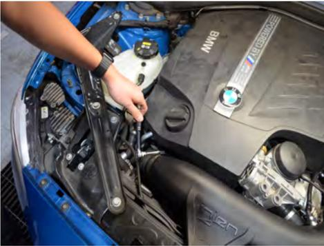
16. Secure the clamp on the turbo inlet pipe.
