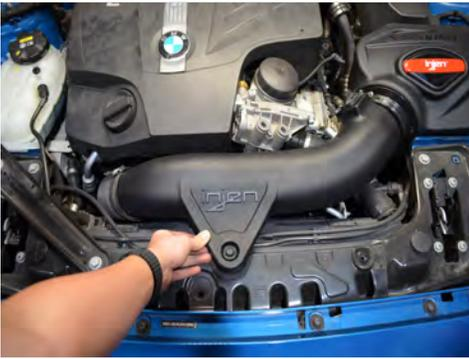
13. Press the injen tube into the turbo inlet pipe. Next press the tube into the twist lock filter. Finally line up the grommet to the stud and press down on the tube.
