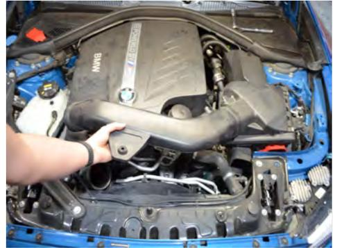
6. Remove the OEM intake assembly.
