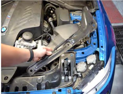
5. *IF EQUIPPED:* Remove the strut tower brace.
