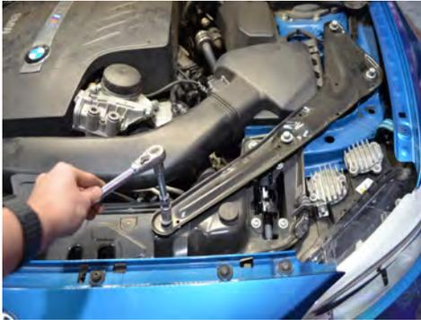
4. *IF EQUIPPED:* Remove the four bolts holding the strut tower brace.
