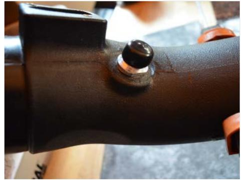
15. If not equipped with crank case line. Cap the crank case fitting with the 3/4" vinyl cap
