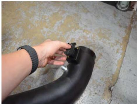
8. Install the MAF sensor into the Injen tube and secure using the provided M4 x 0.7 button head screws.
