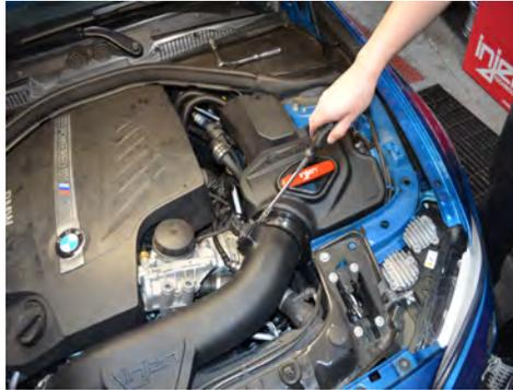
17. Secure the clamp on the twist lock filter.
