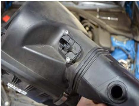
7. Remove the two screws holding the MAF sensor and then remove the MAF sensor.
