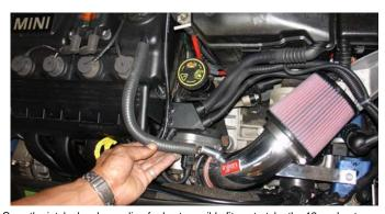
Once the intake has been align for best possible fitment, take the 12mm heat hose and press one end over the crankcase port.
