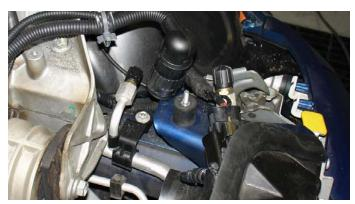
Screw the vibra-mount into the brace until it bottoms out.
