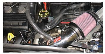
Press the other end of the 12mm heater hose over the intake port(A). Once again align the entire intake for best possible fit then continue to tighten the flange nut on the vibra-mount(B).
