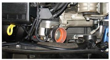
Take the short  $2\ 1/2$ " x  $2\ 3/4$ " step hose and press the  $2\ 1/2$ " end over the throttle body . Use one medium clamp and one small clamp. Tighten the clamp on the throttle body side at this point.
