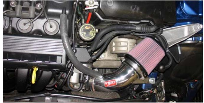
The installation is now complete. Check the entire intake to make sure there are no rubbing parts along the length of the intake then continue to tighten all nuts, bolts and clamps. Failure to check the intake periodically will void the warranty if any damage is caused to the intake.
