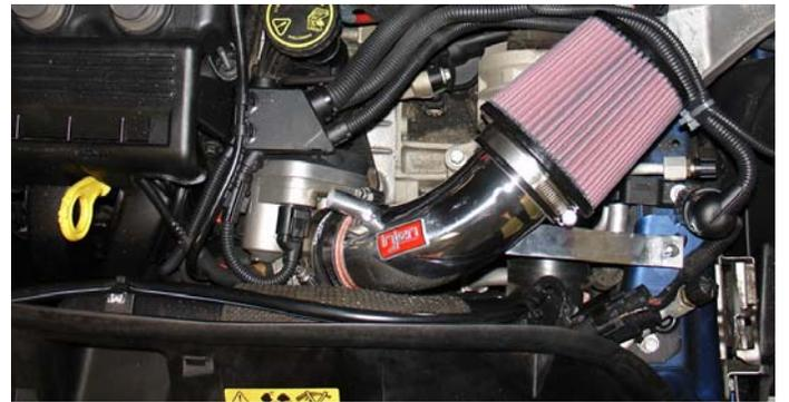
Position the assembled intake and filter into the step hose located on the throttle body. Align the intake for best possible fit. While the intake is positioned, place the bracket on the intake over the vibra-mount stud.
