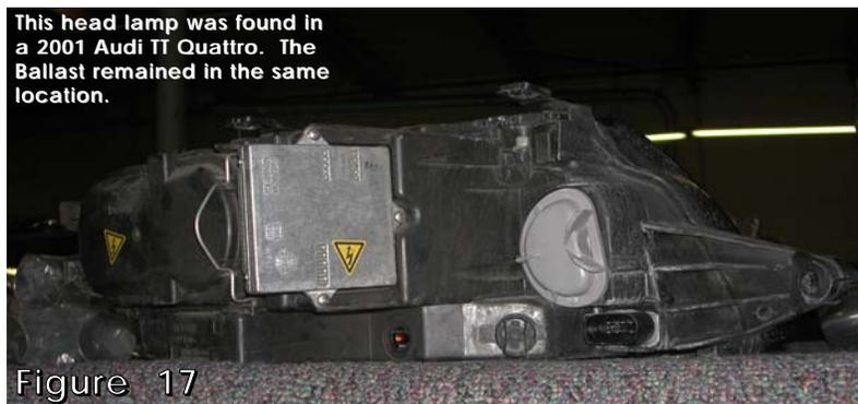
Late models such as this one has the HID ballast built into the head lamp.
