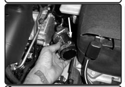
**8.** Loosen the hose on turbo and remove.
