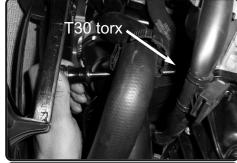
23. Disconnect any lines attached to the cold side intercooler pipe. Loosen the T30 bolt holding in the intercooler pipe.
