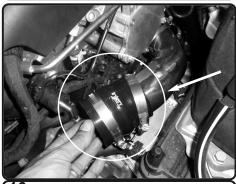
**16.** Install the upper intercooler pipe to the hose on the turbo adaptor. Attach the provided 2-1/2" hump hose with clamps to the upper intercooler pipe.
