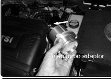
**11.** Once o-ring is installed. Install the new injen turbo adaptor to the vehicle.
