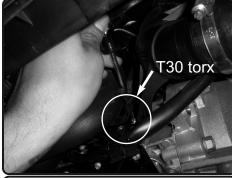
**3.** Loosen the T30 bolt holding in the intercooler pipe on the bottom of the pipe.
