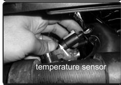
**31.** Re-connect the temperature sensor harness.
