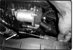
**33.** Install the 2-5/8" hump hose to the throttle body with clamps provided. Connect the hose and adjust. Make sure the hoses are properly adjusted and clamps are behind the bead. This will prevent hoses popping off the pipe
