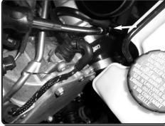
**15.** Secure and tighten on the turbo adaptor only using 8mm nut driver.
