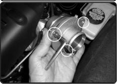
**9.** Loosen the 3 bolts holding in the OEM turbo adaptor using 5 mm allen key. Save the 3 bolts for later install
