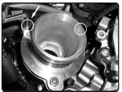
12. Secure the adaptor using original screws from step 9.
