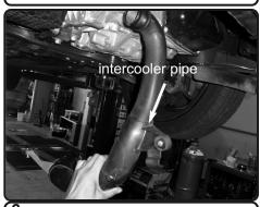
**6.** Carefully pull all harness and lines away from the intercooler pipe. Now remove the hot side of the intercooler pipe out of vehicle.
