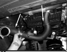
**25.** Carefully pull out the intercooler pipe from the vehicle.
