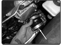
**14.** Install the provided 2-1/2" hump hose with clamps to the turbo adaptor.
