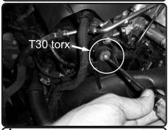
**4.** Loosen the T30 torx bolt on top of the intercooler pipe.
