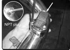
**27.** Install the Temperature sensor into the new intercooler pipe and tighten using provided socket cap screws. Secure the NPT fitting using provided thredded cap if not using for any accessories.
