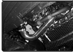
**35.** Secure and tighten clamps using 8mm nut driver. Re-install guard, and intake system. Your intercooler pipe kit is now complete.
