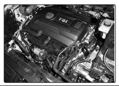
Congratulations! You have just completed the installation of this intercooler pipe system. Periodically, check the alignment of the intercooler pipes, normal wear and tear can cause nuts and bolts to come loose. Note: Check clearance and adjust if needed! Failure to check the alignment and adjust the intercooler pipes can cause damage that will void the warranty. Injen Technology is not responsible for any damages caused by/from improper installation.
