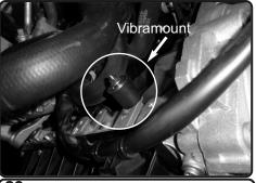
**29.** Install the vibramount to the original mounting location from step 23. Secure and tighten.
