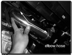
18. Install the lower intercooler pipe into the vehicle. Position to the upper intercooler pipe and bracket to the vibramount.
