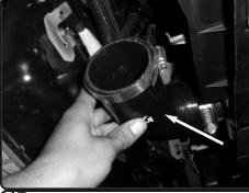
Install the elbow hose to the intercooler, short side first with clamps provided. Do not tighten .
