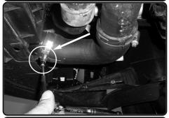
**22.** Loosen the clamp on intercooler using 7mm nut driver or wrench.
