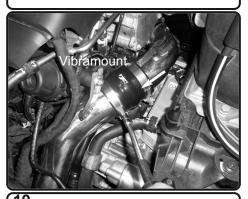
Connect the hose and adjust. Make sure the hoses are properly adjusted and clamps are behind the bead. This will prevent hoses popping off the pipe. Secure the bracket using provided washer
