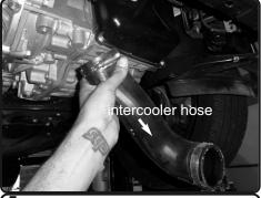
**5.** Remove the lower intercooler hose. Loosen the clamp on top of the turbo side using 7mm nut driver.
