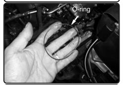
10. Check and verify the o-ring did not fall out, if so. use some grease and re-install to the groove cut out on the turbo. The grease will keep it from falling off.
