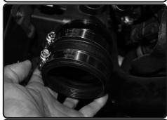
**9.** Install the provided step hose with clamps to the turbo.
