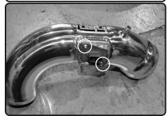
**8.** Install the MAF sensor in the correct direction. Secure using the provided M4 screws. Tighten using 2.5mm allen key.
