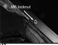
17. Secure and tighten the bottom of the heatshield using provided M6 lock nut. Secure and tighten using 10mm socket or wrench.
