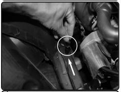
**4.** Carefully lift up and remove the entire stock air box assembly.
