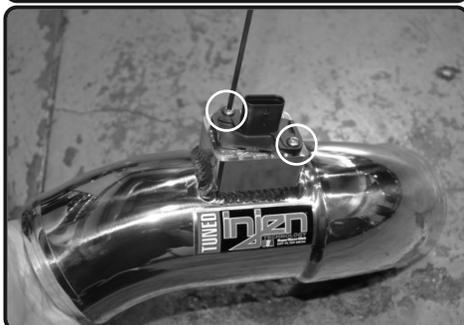
9. Install the MAF sensor in the correct direction. Secure using the provided M4 screws. Tighten using 2.5mm allen key.
