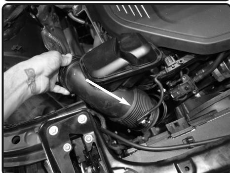
4. Loosen the clamp on the turbo using 7mm nut driver and remove the intake tube out of the vehicle.
