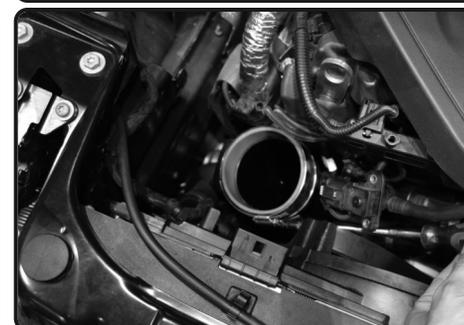
11. Tighten the clamp on the turbo side only using 8mm nut driver.
