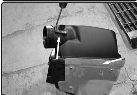
8. Remove the 2 screws holding in the MAF sensor using T25 torx bit.
