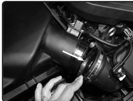
7. Loosen the clamp on air box and pull back the intake tube.
