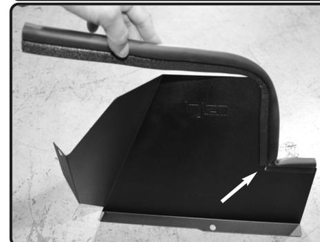
7. Install rubber trim to the top of the heatshield. Notch corner for easier installation.
