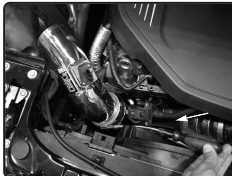
**18.** Install the intake tube and position for the best fit. Tighten clamp using 8mm nut driver.
