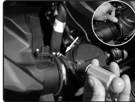
3. Loosen the clamp on the air box using 6mm nut driver. Pull back the intake tube from the air box.
