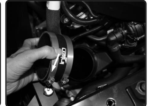
**20.** Install the provided 4" straight hose with clamps to the plastic intake tube. Tighten clamp on the plastic tube only.
