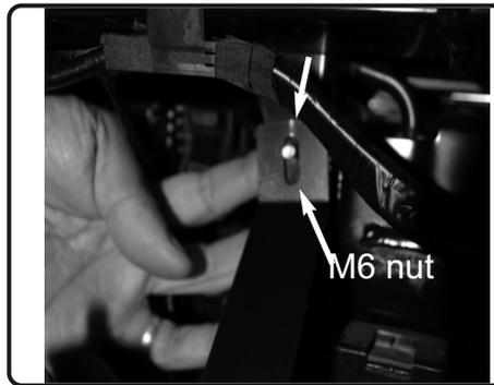
**15.** Secure the heatshield tab to the radiator support using M6 screw and M6 nut. Secure and tighten using 10mm wrench or ratchet.
