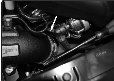
**23.** Tighten the clamp on the intake tube using 8mm nut driver.
