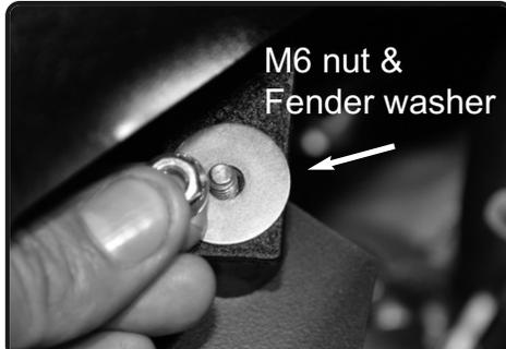
**22.** Secure the bracket on intake tube using provided M6 nut and fender washer. Tighten using 10mm socket or wrench.
