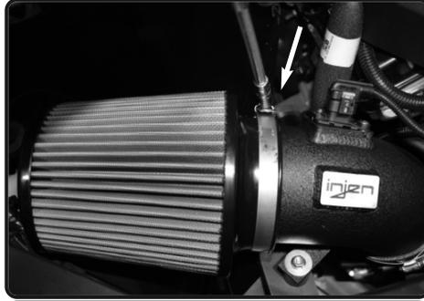
**26.** Secure and tighten using 8mm nut driver. Re-adjust if you need to and re-tighten intake tube.
