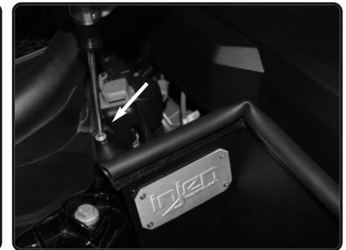
**16.** Secure the tab on heatshield using the OEM torx screw. Secure and tighten.
