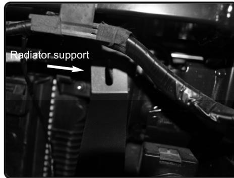
**14.** MAKE sure the heatshield is flat on frame. Locate the hole on the radiator support.
