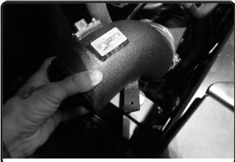
**21.** Install the intake tube into the vehicle and position to the straight hose and bracket to the vibramount.
