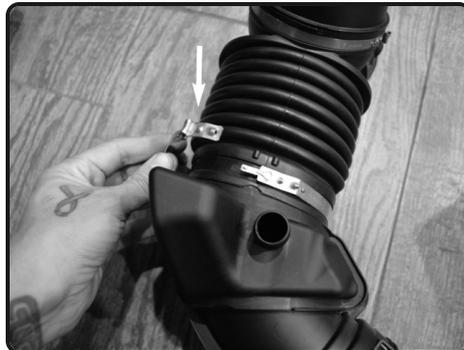
6. Remove the security clamp from intake tube.
