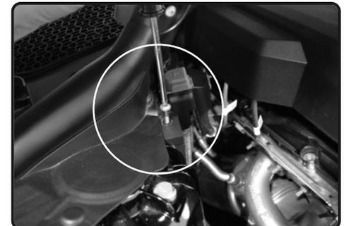
12. Loosen the T30 torx screw located on the frame in front of Plastic ram scoop. Save bolt for later install.
