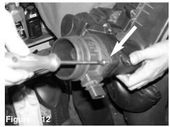
With phillips screwdriver, loosen the 2 screws holding in the MAF sensor.
