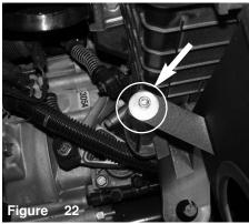
Now secure the tab using provided allen screw and fender washer.
