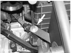
Tighten screw using 6mm allen key.
