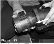
Carefully pull back the MAF sensor from the air box.
