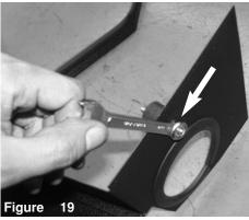
Tighten using 10mm wrench.
