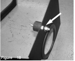
Install the provided vibra mount to the heat shield with vibra mount closes to the engine. Secure using provided me nut
