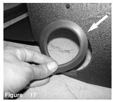
Attach the vinyl trim to the inside of heat shield hole cut out for the intake tube.
