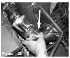
Install the intake tube and position through the hole on the heat shield. Position the bracket to the vibra mount and to the straight hose.
