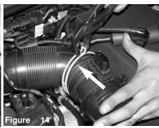
Re-install into the vehicle and secure using factory clamp.
