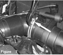
With pliers compress the clamp and pull away.
