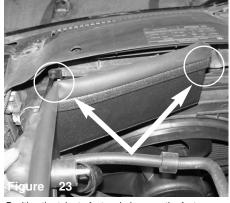
Position the tabs to factory holes, use the factory screws from step 16, secure and tighten.
