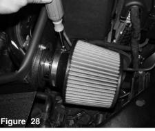
Now install the air filter and tighten using 8mm nut driver. Tighten all clamps using 8mm nut driver. Position for the best fit.
