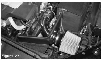
Align for best fit and tighten all clamps. Re-install the engine cover.
