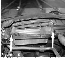
With T25 torx bit loosen the 2 screws holding in the factory ram scoop and remove. Save screws for later install.
