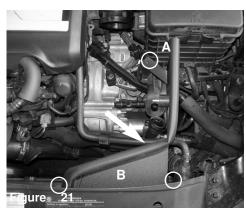
A)Install the heat shield and position the bracket to the original air box screw location. B)Also position the front of the heat shield to the holes from step 16.
