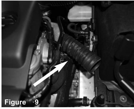
Figure 9 This is an auxiliary heater hose line that picks up ambient warm air on cold starts. This will not be used with the injen intake kit.
