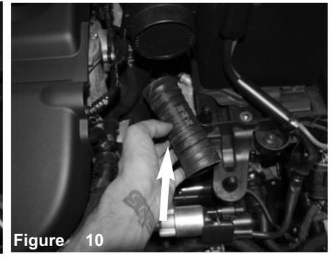
Figure 10 Carefully remove the heater hose from vehicle.
