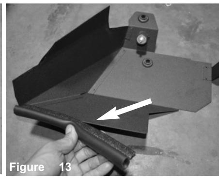
Figure 13 Attach the rubber trim to the heatshield, with pliers or scissors, notch 1 side of the trim for easier fit.
