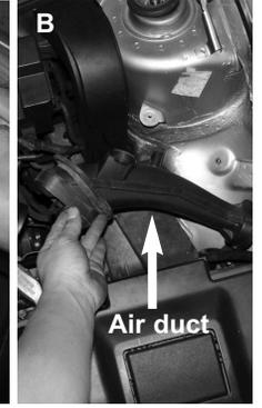
**Figure A:** On the right side of the battery, locate the air box air duct and unbolt the 10mm nut. **Figure B:** Now remove the entire air duct assembly
