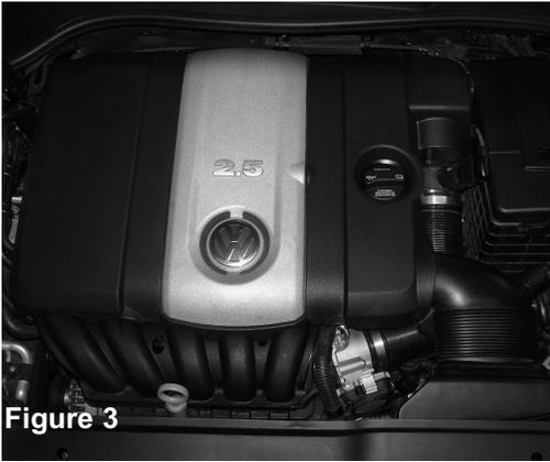
Picture of factory air intake system
