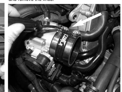
Install the straight hose with clamps to the throttle body. Tighten the clamp on throttle body only using 8mm nut driver.
