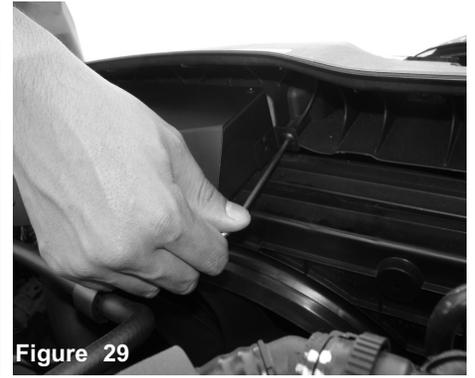
Secure using remaining factory screw.
