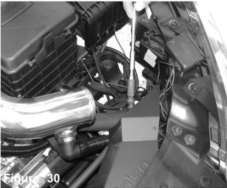
With adjustable torx snake, tighten both screws.
