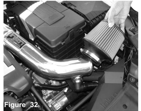
Install the filter and secure using 8mm nut driver.
