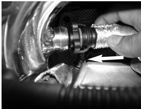
Connect crank case line to intake tube.
