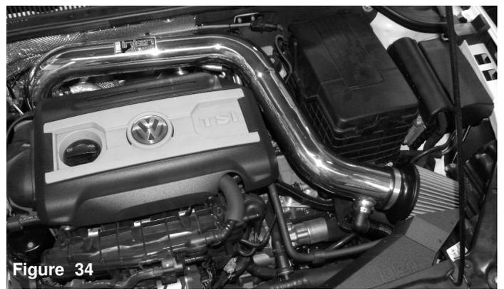
Figure 34 Congratulations! You have just completed the installation of this intake system. Periodically, check the alignment of the intake, normal wear and tear can cause nuts and bolts to come loose. Failure to check the alignment and adjust the intake can cause damage that will void the warranty.
