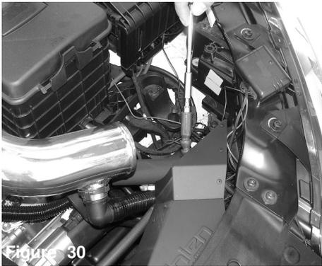
Figure 30 With adjustable torx snake, tighten both screws.
