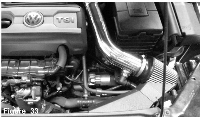
Figure 33 Image of the filter and power-ram unit.
