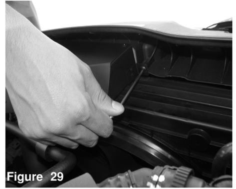
Figure 29 Secure using remaining factory screw.
