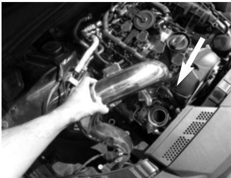
Install the intake tube into vehicle.
