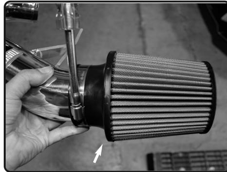
**13.** Secure and tighten using 8mm nut driver.
