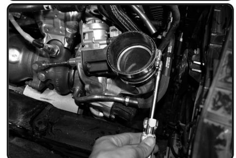
11. Tighten the clamp on turbo only.
