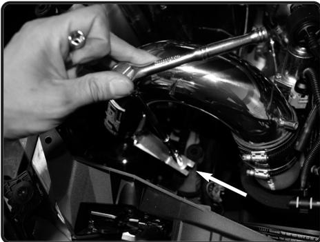
**16.** Tighten bracket using 10mm socket or wrench.
