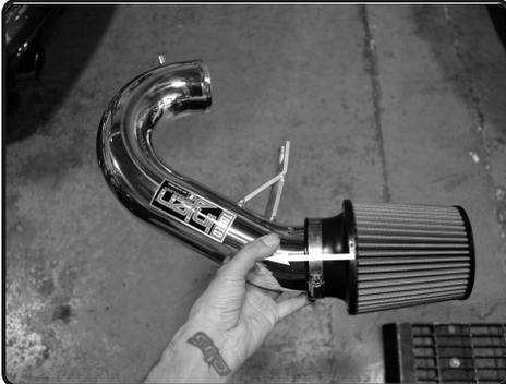
**12.** Install the filter to the tube.
