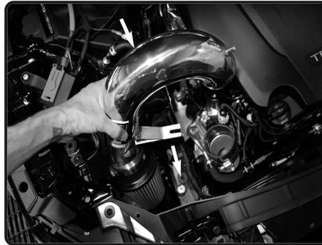
**14.** Install the intake assembly into the vehicle.
