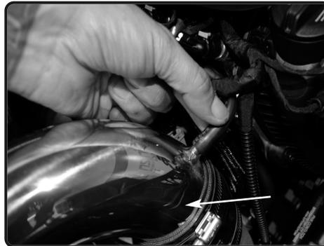
**18.** Connect the vacuum line to the fitting on the intake tube.
