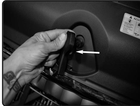
7. Carefully remove the lever out of vehicle,
