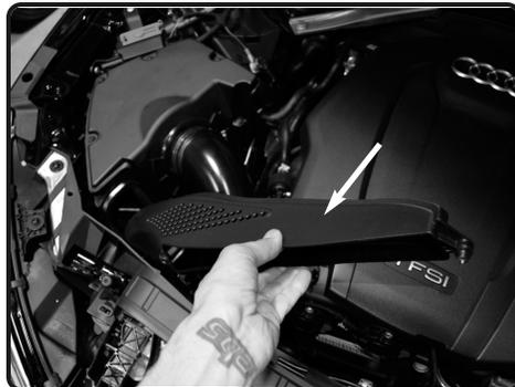
5. Remove the ram scoop from vehicle.
