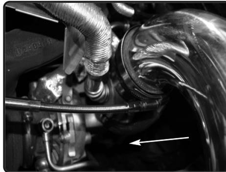
**19.** Secure the hose and tighten using 8mm nut driver.
