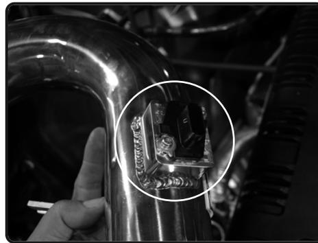
**14.** Install the MAF sensor into the new intake tube in correct direction, secure and tighten using OEM screw and tighten.
