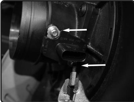
**13.** With provided T20 torx security bit, loosen and remove MAF sensor. Save screws for later install. **Note: Keep sensor in same direction.**
