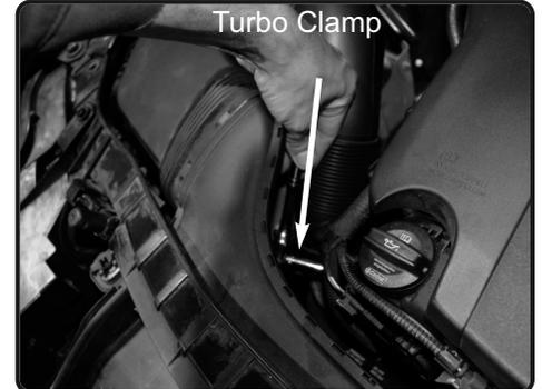
8. Loosen the clamp on the turbo using 7mm socket with ratchet.
