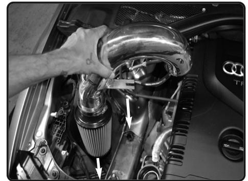
**16.** Install the intake tube assembly. position the bracket to the washer and the intake tube to the step hose.
