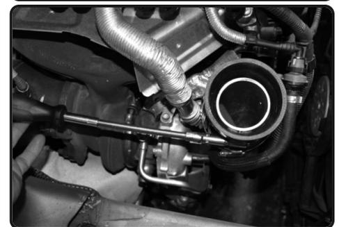
12. Tighten the clamp on turbo only.
