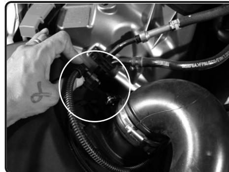
7. Disconnect the MAF sensor harness from the intake tube. Pull
