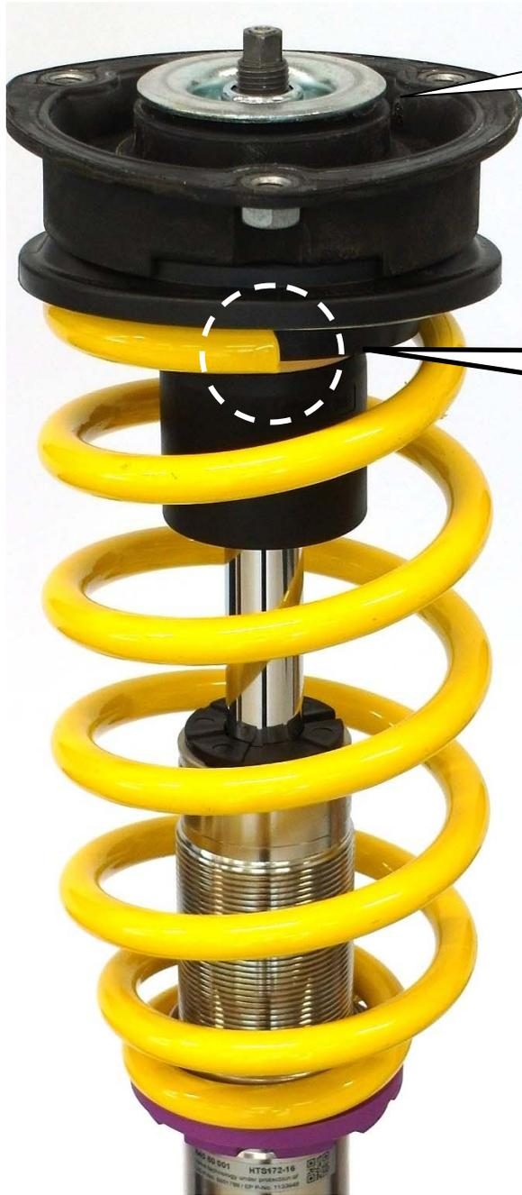
Attach the original top mount and fix it with the supplied nut. Tightening torque for the piston rod is 50 Nm (37 ft-lb). Please install the strut unit to manufacturers recommended settings regarding tightening torque and fixing specifications.
