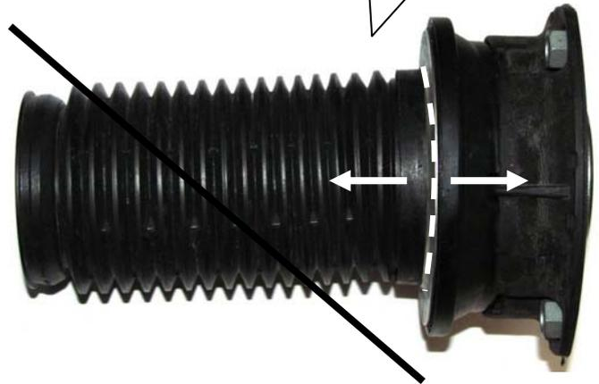
The marks of the OEM upper top mount (upper part) and the OEM axial bearing (bottom part) need to be put on top of each other! The marks show to the vehicle internal side in installed condition.
