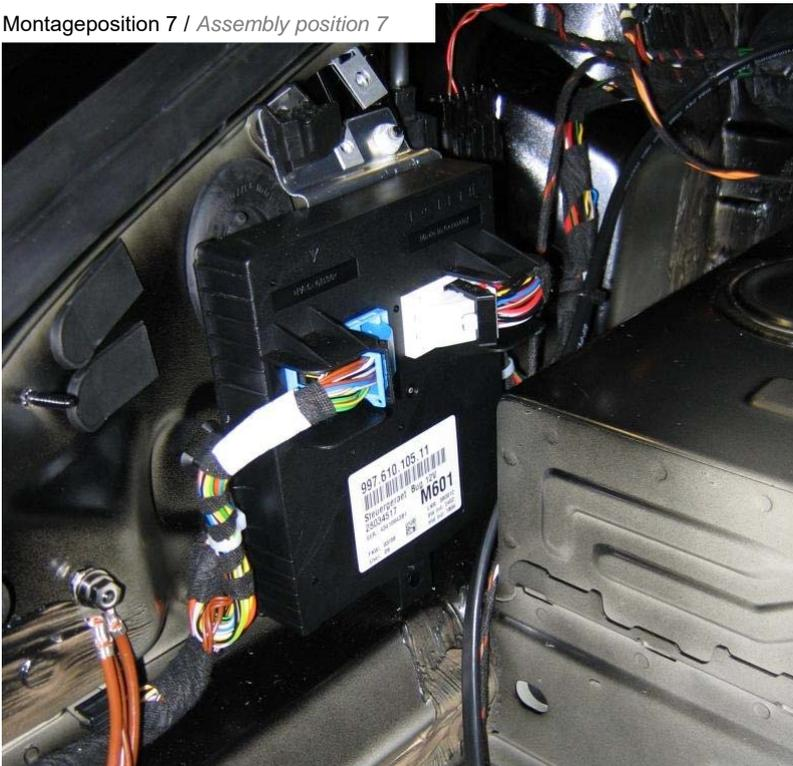
**Anschluss Innenraumtaster / *Connection the Interior cabin button***
