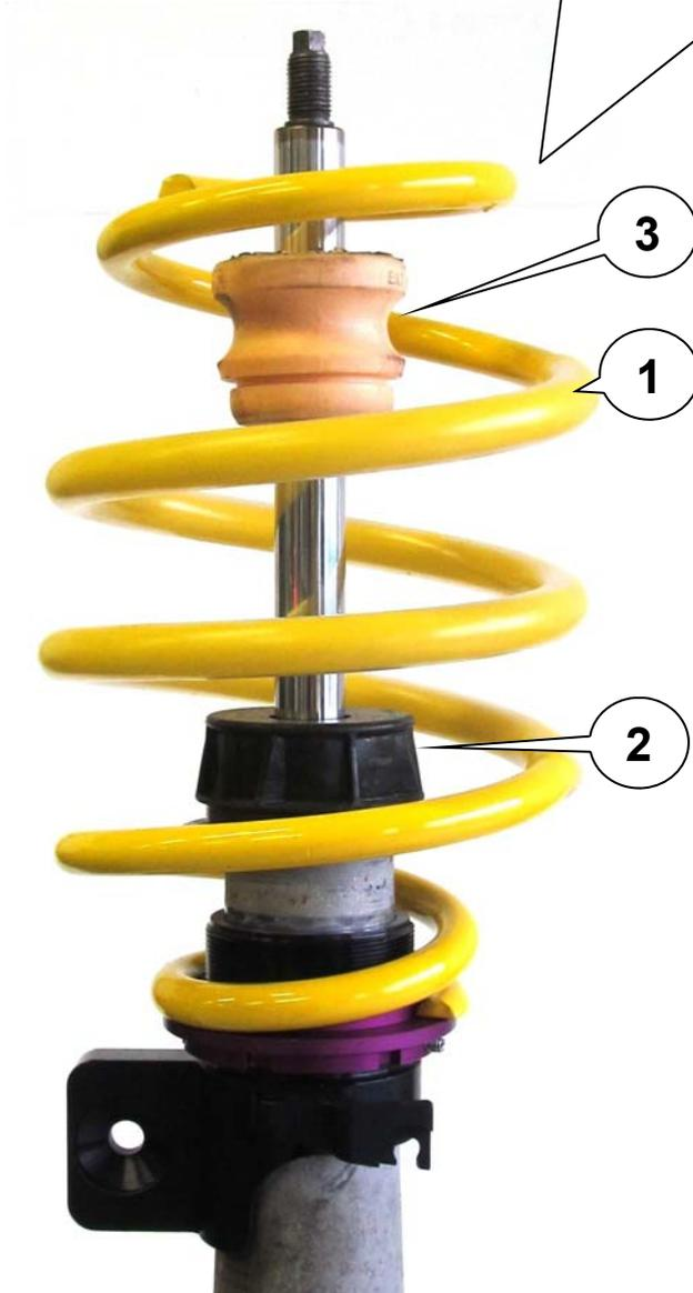
Install the OEM supporting bearing with dust cover and fix it with the standard nut. Please install the strut unit to manufacturers recommended settings regarding tightening torque and fixing specifications.
