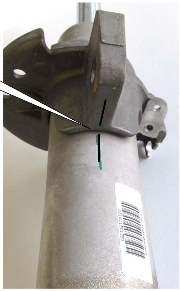
Detach the standard ventilation disk on the sway bar holder from the coilover strut.
