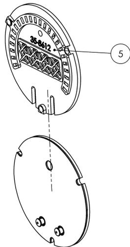
STEP 3 - Slide the light guide (5) upward to remove it, the buttons may fall out at this time - take care not to lose them
