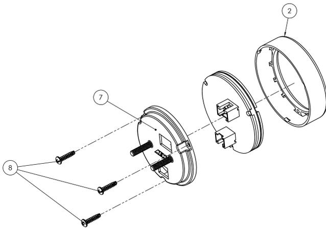
STEP 1 - Remove the three assembly screws (8) using a #1 Phillips head screwdriver. Separate the bezel (2) and cup (7) from the rest of the assembly. If you have purchased the optional accessory kit, the silver bezel may be replaced for the existing bezel at this time
