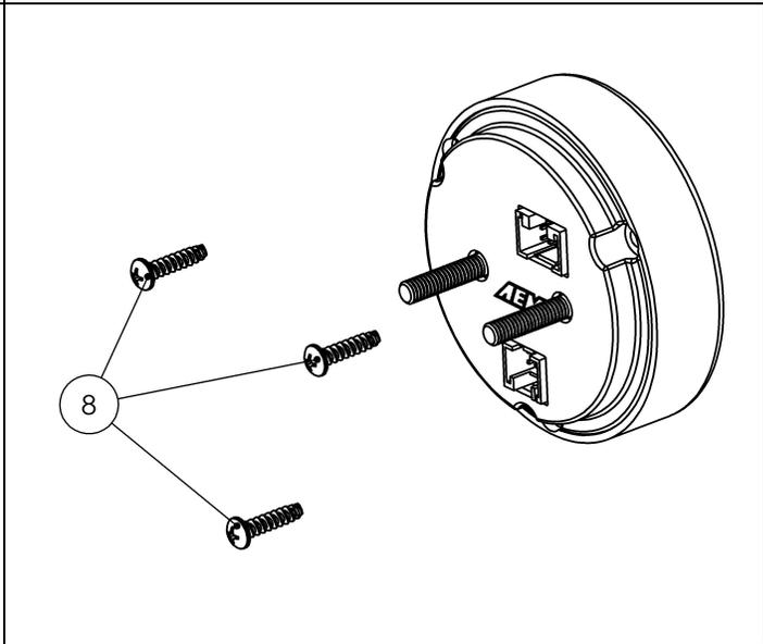
STEP 4 - Reassemble and tighten screws to 2 in-lb (previously assembled bezel) or 3 in-lb (new bezel). Do not over-tighten!
