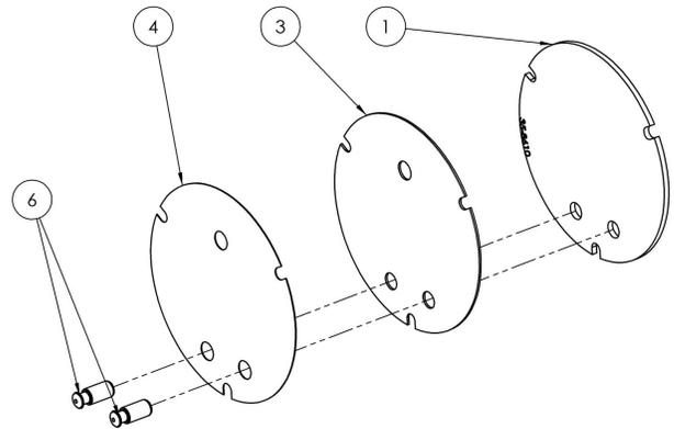
STEP 4 - As you separate the remaining components, diffuser (4), faceplate (3), lens (1), note the order in which they were assembled. The faceplate (3) may now be reversed to display an alternate scaling or replaced for a different color as included in the optional accessory kit
