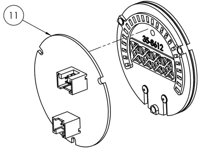
**STEP 2** - Separate the PCB (11) from the remaining components
