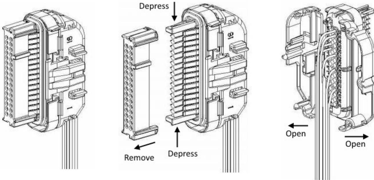
The clear retainer will have to be removed to insert/remove pins
