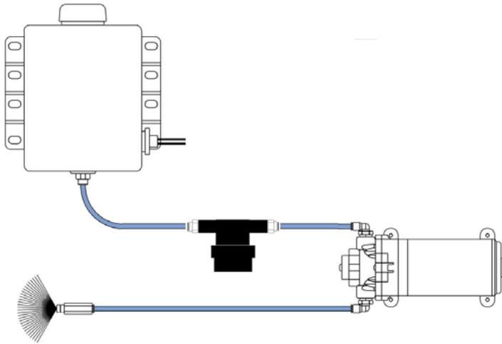
1. Install filter on the low pressure side between the tank and pump. Splice into existing line by cutting tubing with a sharp razor blade. Install filter with arrow on housing pointing in the direction of flow.
