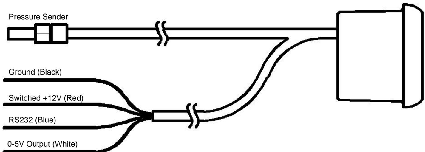
Figure 1. Connection Diagram
