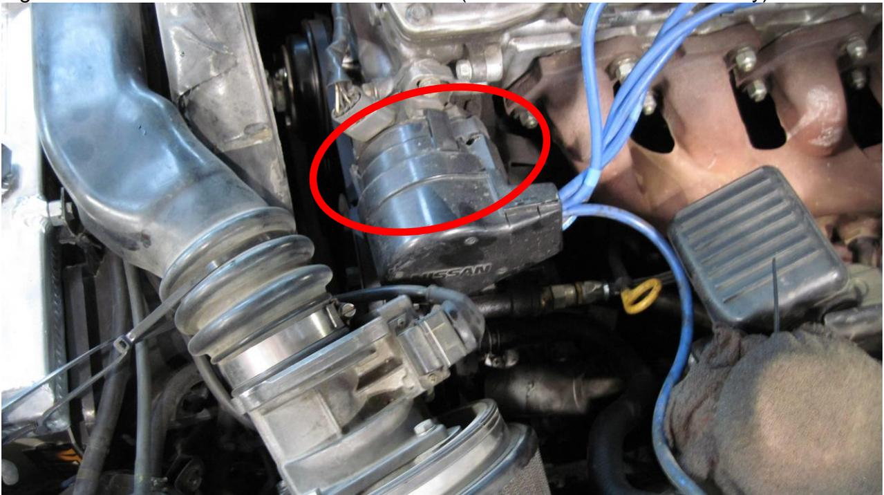
Figure 2: Location of CAS sensor (underneath distributor cap)
