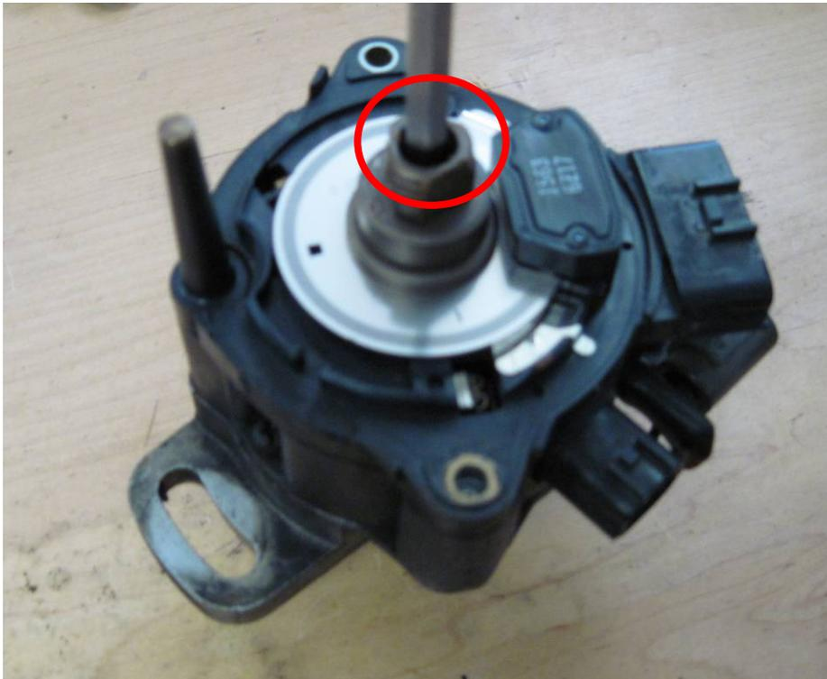
Figure 4: Removal of screw holding on CAS disc
