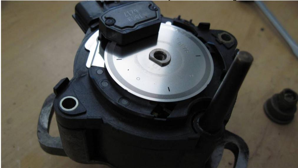
Figure 5: Original CAS screw and collar removed
