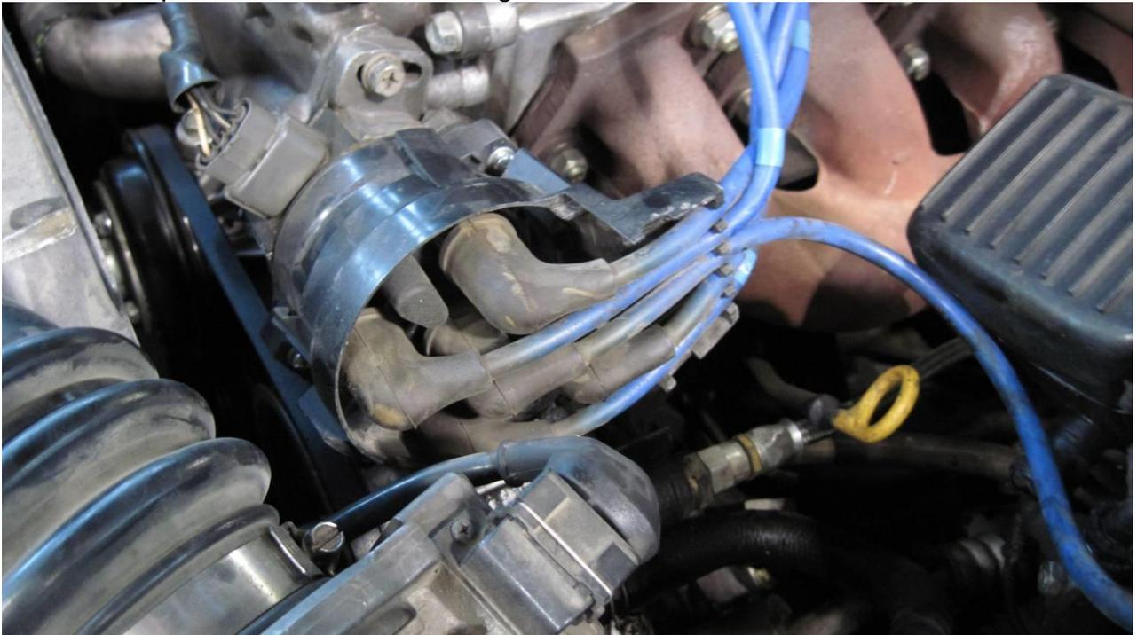
Figure 3: Plastic wire cover removed
