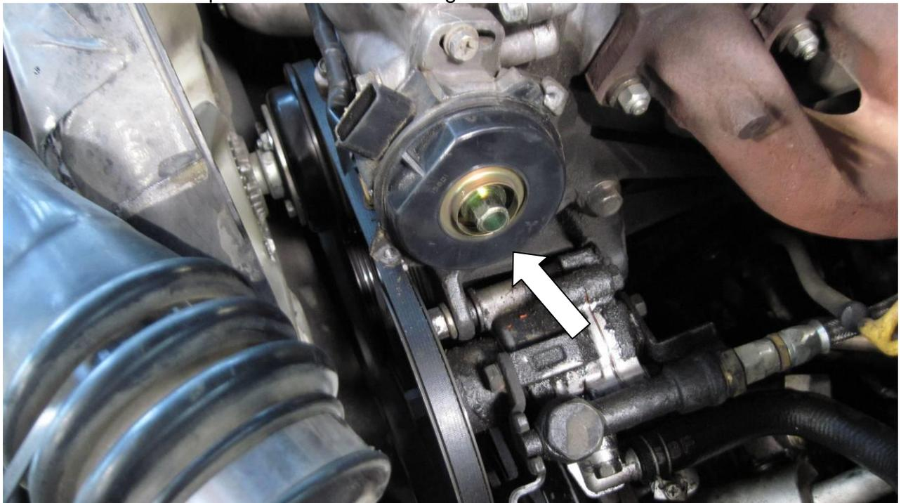
Figure 6: Internal plastic cover to be removed
