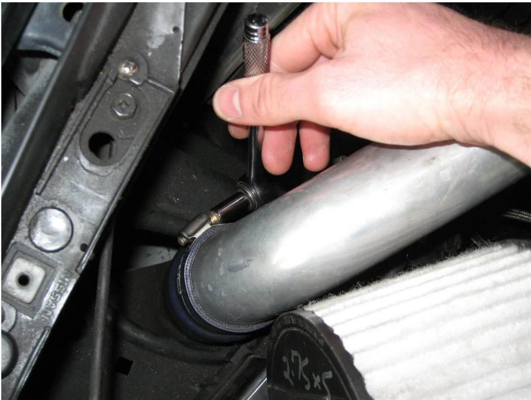
Figure 5: Removal of intake tube
