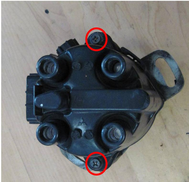
Figure 1: Distributor cap removal
