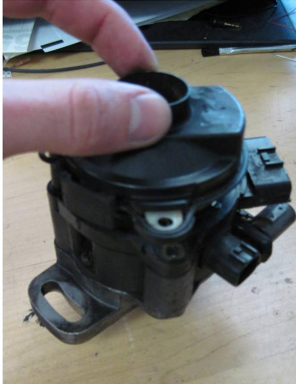
Figure 3: Removal of internal cover over CAS disc
