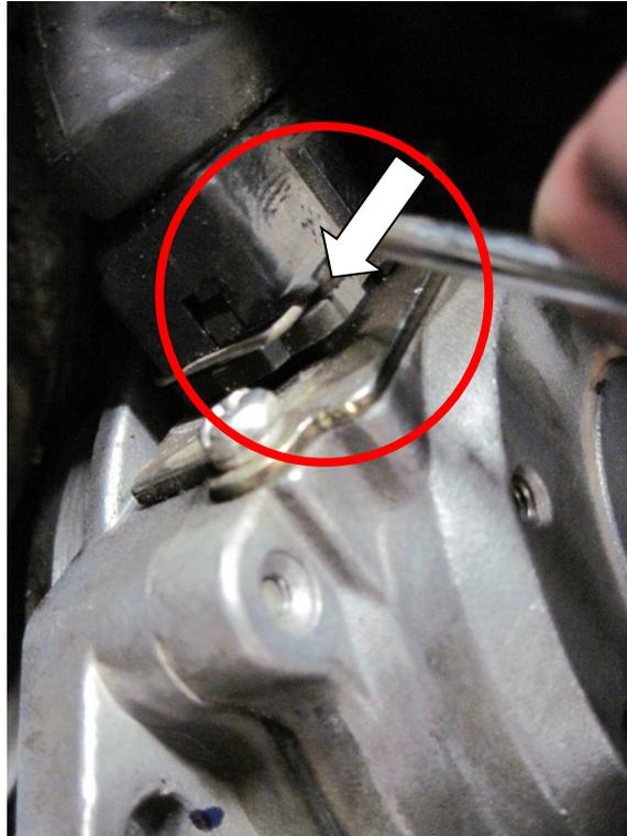
Figure 9: Pry here to remove this clip
