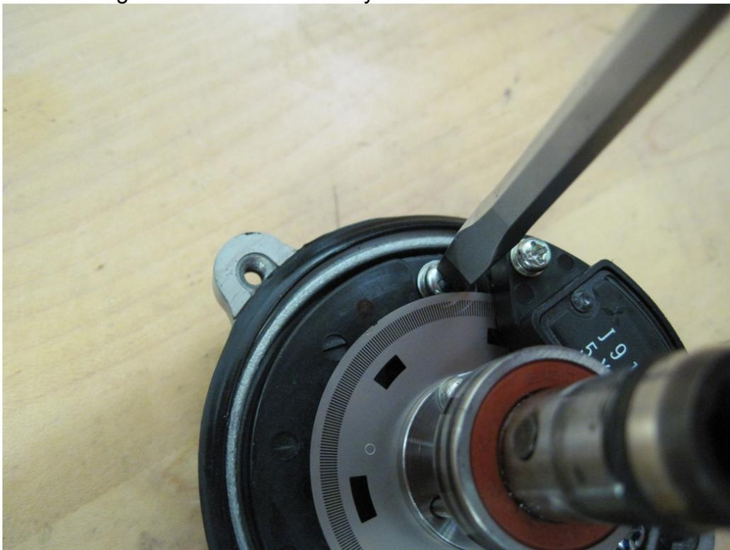
Figure 18: Remove 3 screws holding sensor using 1/4" flat screwdriver
