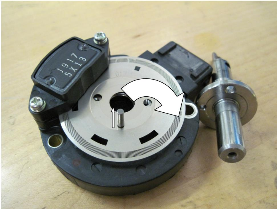
Figure 31: CAS disc screws and shaft removed
