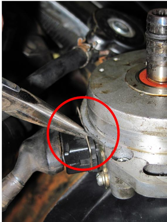
Figure 10: Remove clip with needle-nose pliers
