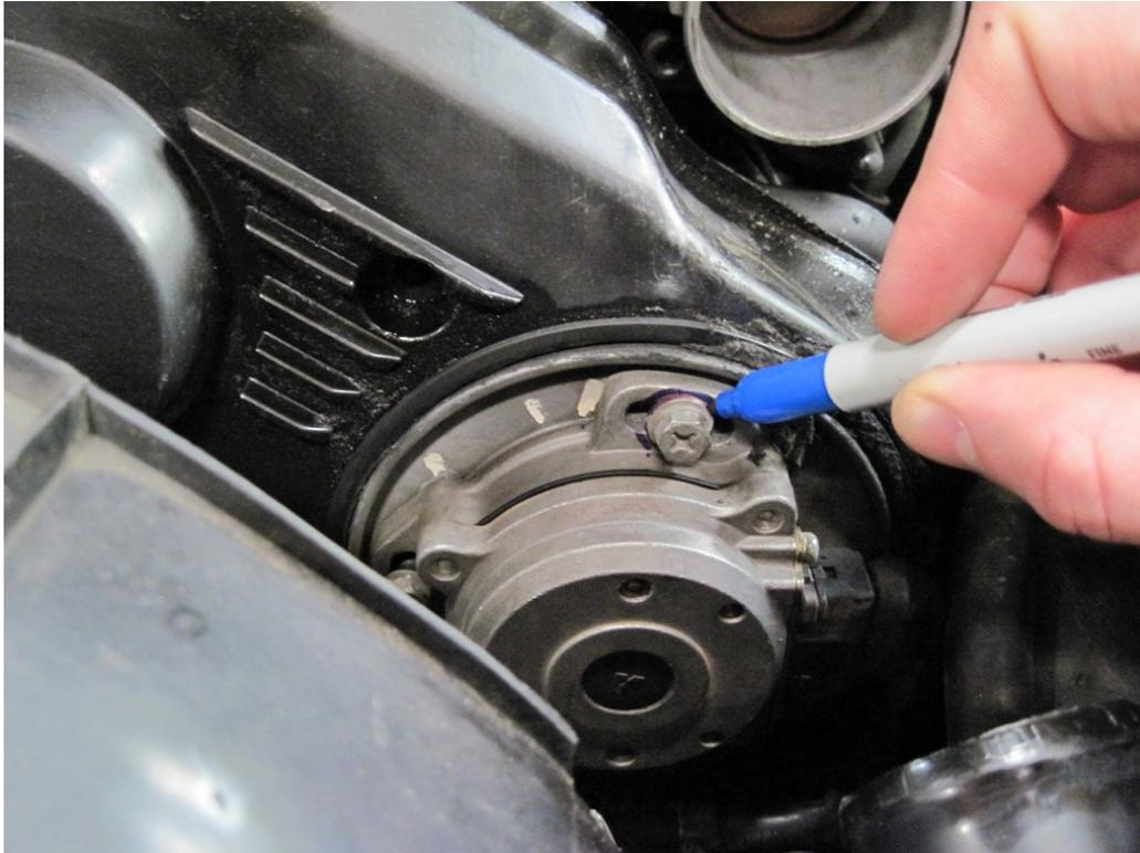
Figure 7: Marking position of CAS sensor
