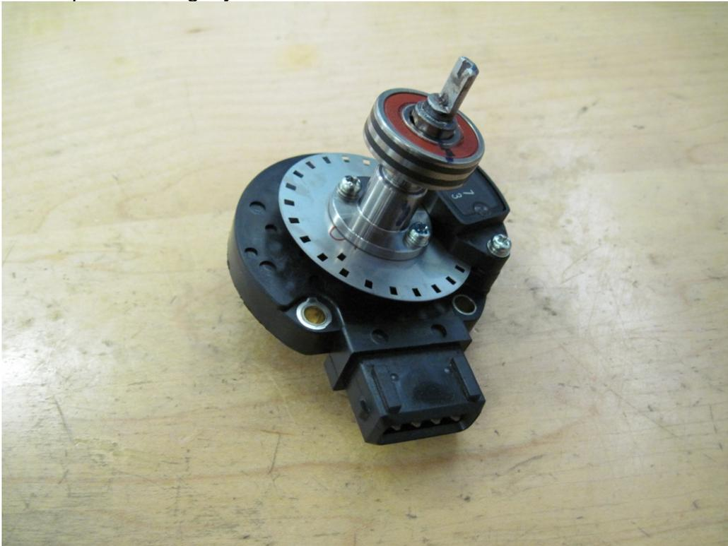
Figure 36: Bearing placement on CAS shaft
