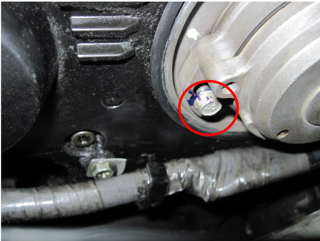
Figure 8: Marking position of CAS sensor
