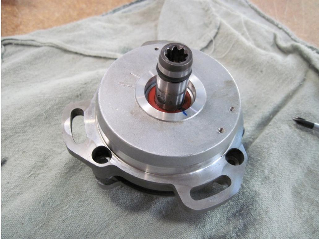
Figure 41: Housing cover reinstalled
