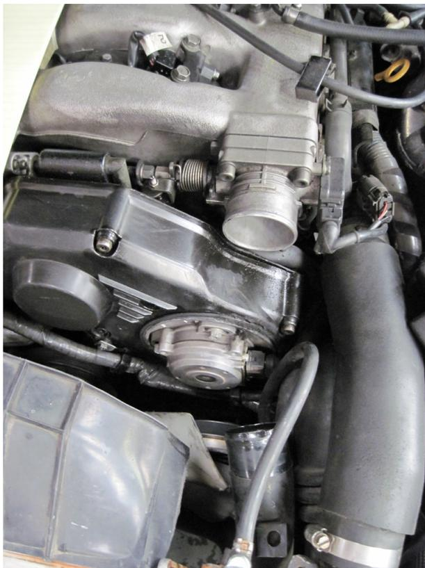
Figure 6: Intake tube removed to access CAS sensor
