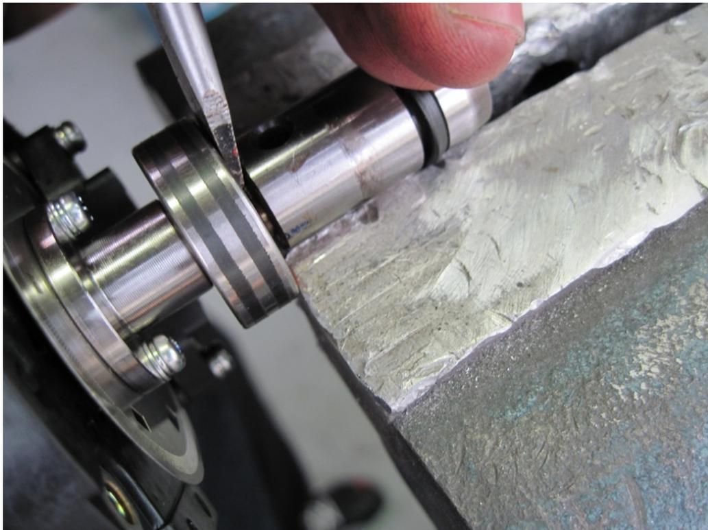
Figure 26: Removal of star socket using 1/4" flat screwdriver
