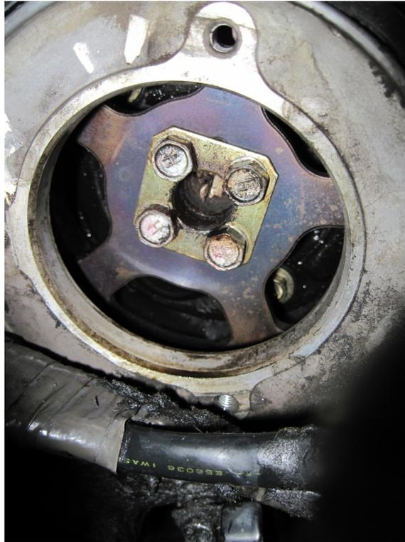
Figure 13: CAS sensor removed
