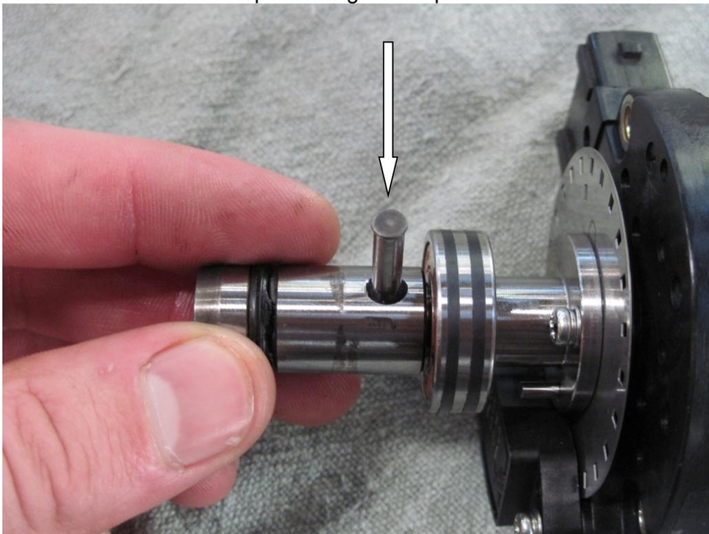
Figure 38: Aligning the star socket retaining pin
