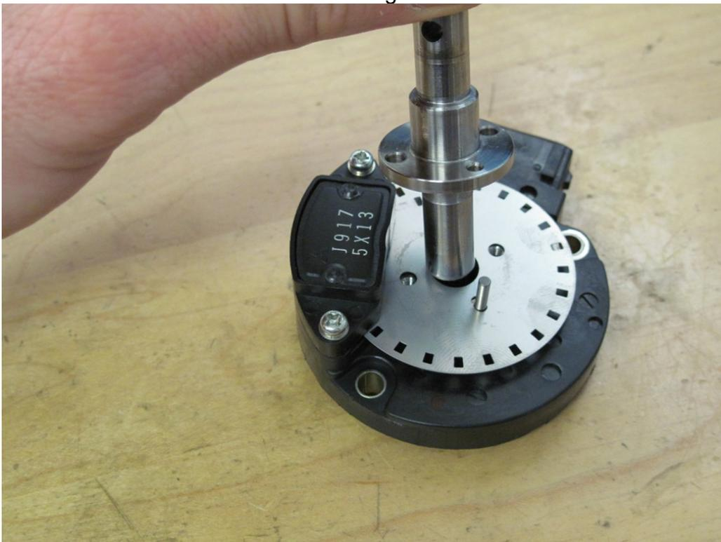
Figure 34: CAS sensor shaft reinstallation
