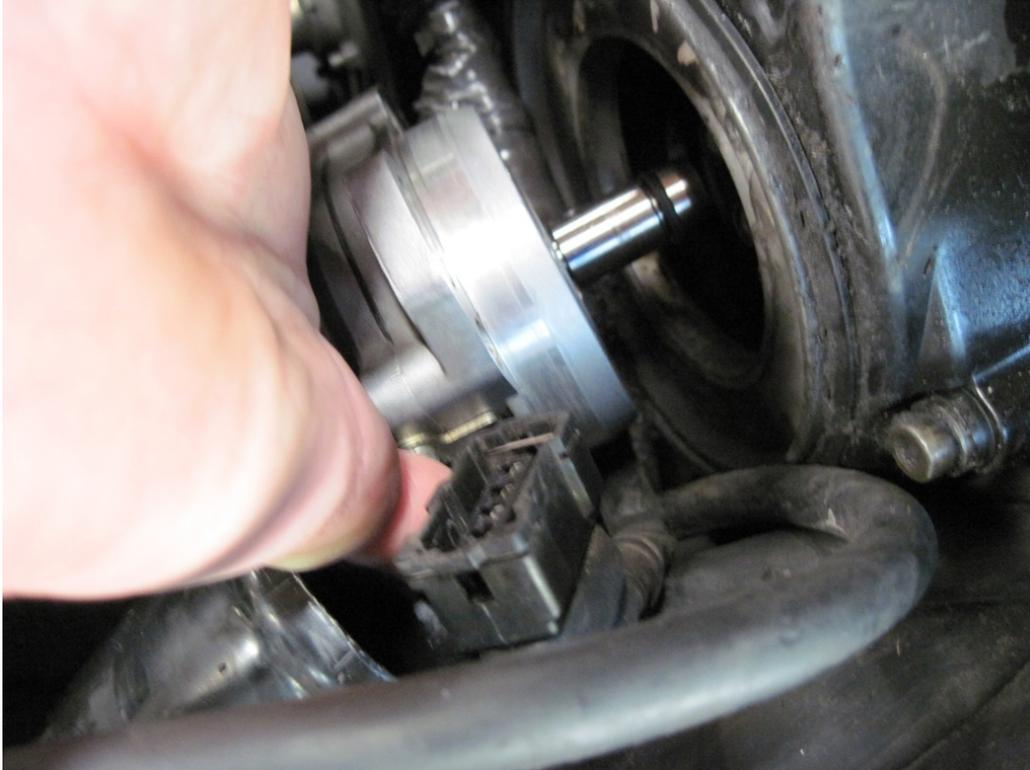
Figure 43: Reinstalling the CAS sensor
