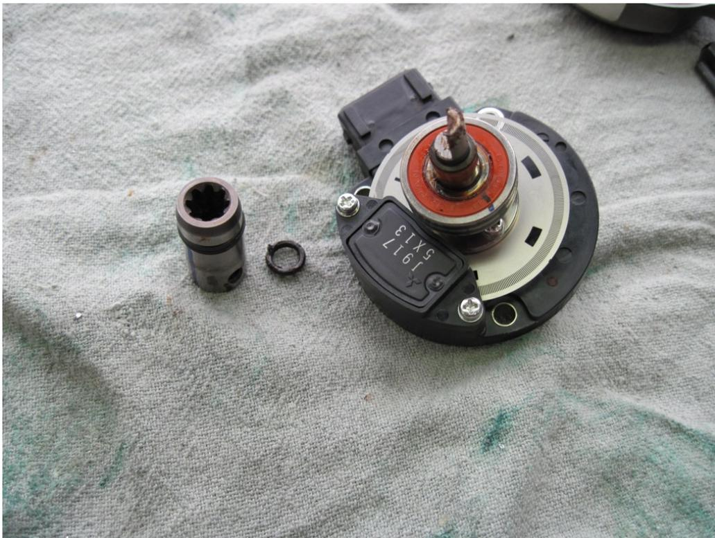
Figure 27: Star socket removed from CAS sensor
