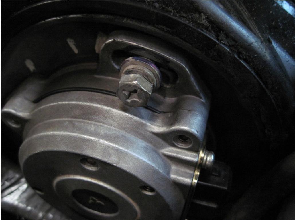
Figure 44: Reinstalling CAS sensor bolts
