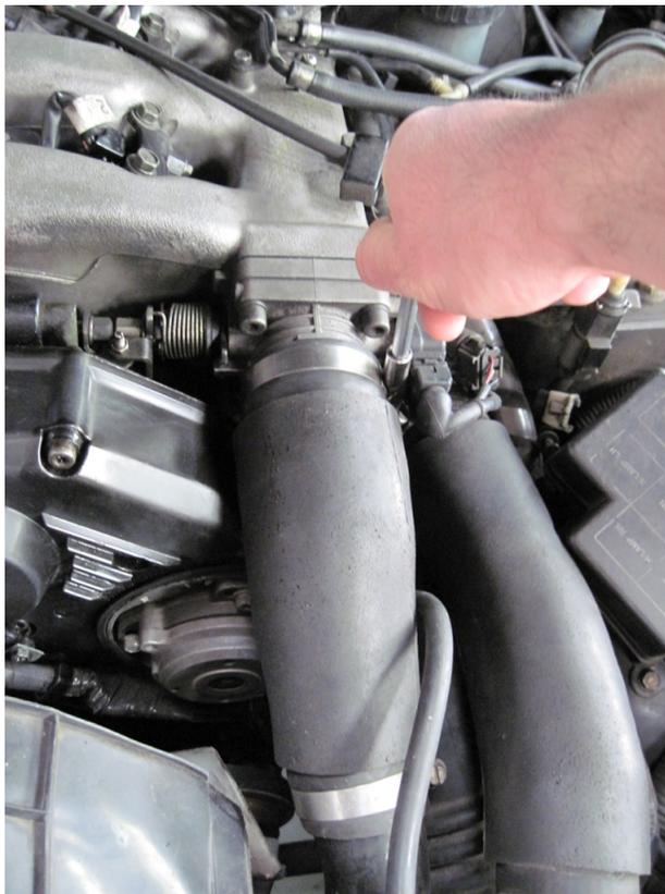
Figure 5: Removal of intake tube using 8mm socket
