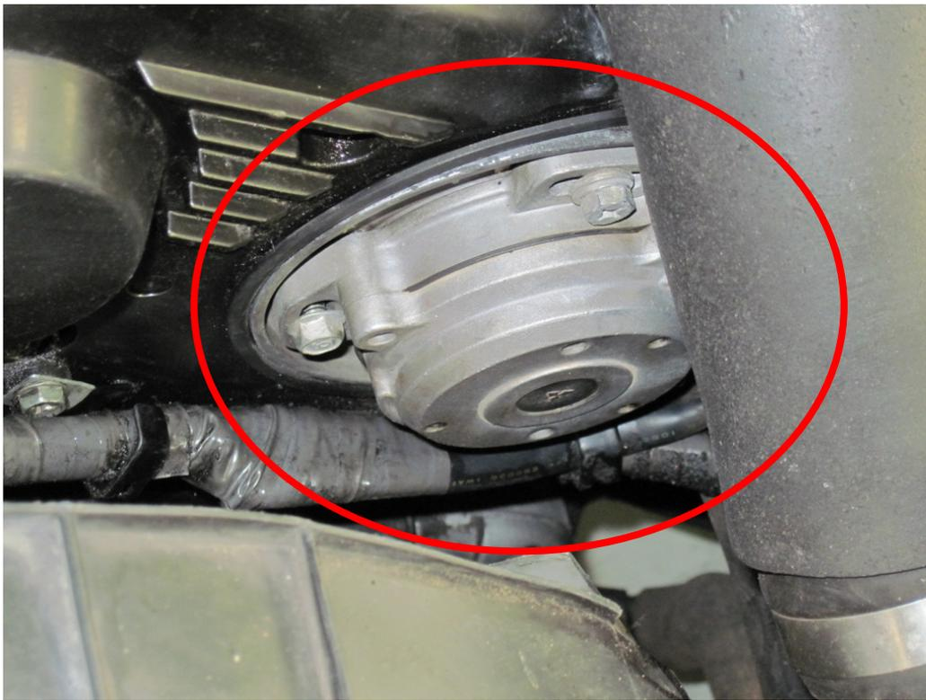
Figure 3: Close-up of CAS sensor
