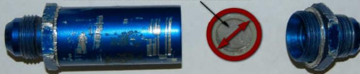
Off-brand "100-micron filter", returned with an A1000 pump the customer claimed was defective... is it any mystery why the pump failed to perform? Nope!!
