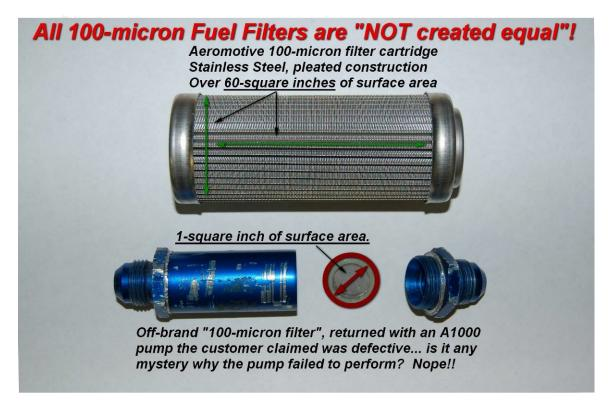
You may run any brand of filter you choose on your car, just be certain that it meets the following requirements: *The filter element used on the inlet side of any Aeromotive fuel pump may be no finer than 100-micron (no number smaller than 100), with a surface area of 60 square inches or more.*
