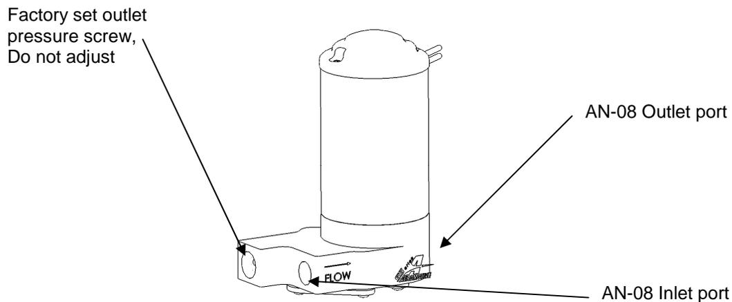
5. Connect the fuel tank or cell to the high capacity 100 micron filter, using an AN-06, AN-08 or equivalently sized fuel line. Connect the filter outlet to the fuel pump inlet (see Flow arrow on pump). These sections of fuel line should be as large a diameter and short as possible to reduce the tendencies for vapor lock, cavitation, and premature wear of your Aeromotive fuel pump.
