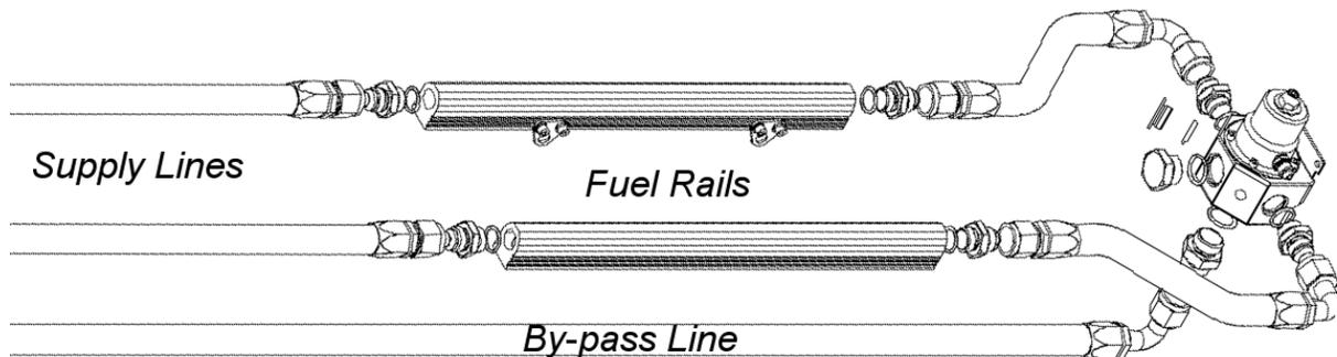
5. Using a Y-block, split the supply line into two AN-08 lines and feed one side of each fuel rail. From the other end of each fuel rail run an AN-08 line into each of the AN-08 ports on the regulator using the two supplied AN-08 fittings and o-rings.
