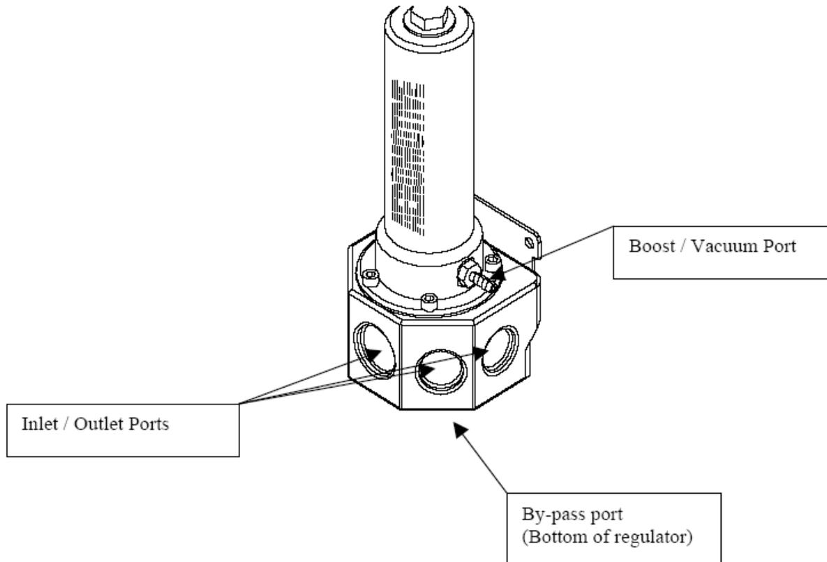
7. Attach the fuel return line to the AN-10 bypass port located at the bottom of the regulator using a cutoff AN-10 style fitting and o-ring. The typical fittings used are as follows; Aeromotive P/N 15608 (AN-10 Port to AN-10 flare) or P/N 15642 (AN-10 Port to AN-12 flare).
