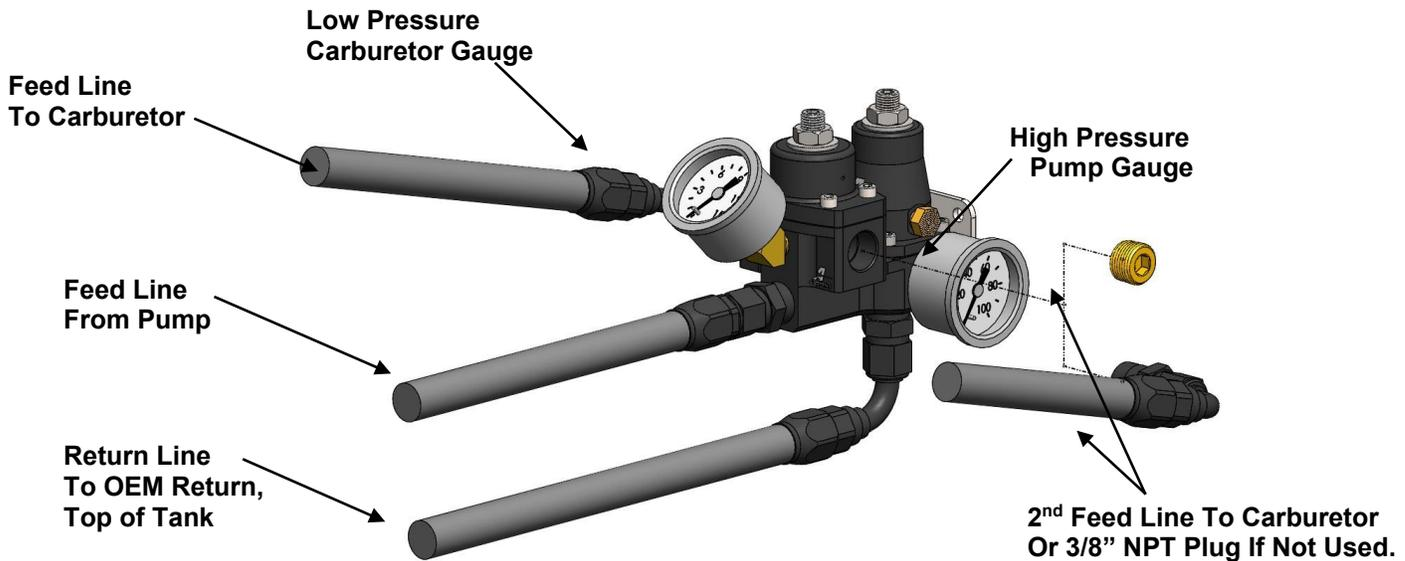
11. Install a suitable high pressure gauge in one of the 1/8" NPT high pressure gauge ports on either side of the pump regulator (Aeromotive P/N 15633, 0-100 psi gauge). Install the included 45-degree, 1/8" NPT street elbow into the 1/8" NPT low pressure gauge port in the front of the carb regulator and then the low pressure gauge into the street elbow. (Aeromotive P/N 15632, 0-15 psi gauge). Gauge connections require appropriate thread sealant such as Loctite 565 or equivalent.
