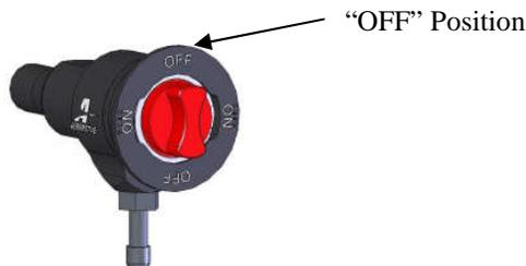
7. When a fuel sample is needed, rotate the red locking knob to the "ON" or unlocked position and press the knob until the desired sample is acquired. After the desired sample has been taken return the red locking knob to the "OFF" or locked position.
