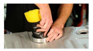
25. NOTE: COMPLETE THIS STEP ONLY IF YOU PLAN ON USING A RETURNLESS FUEL SYSTEM where the ECU uses PWM to control fuel pressure. In this case you must drill a 1/32" hole thru the pipe plug indicated below. If you are planning on using a traditional, return style fuel system please skip this step If you are unsure what your system requires, please contact your EFI system manufacturer or Aeromotive for assistance.
