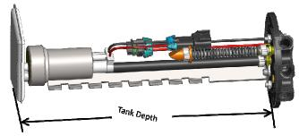
Note: Failure to position the fuel pump strainer on the bottom of the basket assembly will potentially starve the pump for fuel when fuel tank level is low, yielding poor drivability and reduced pump performance.
