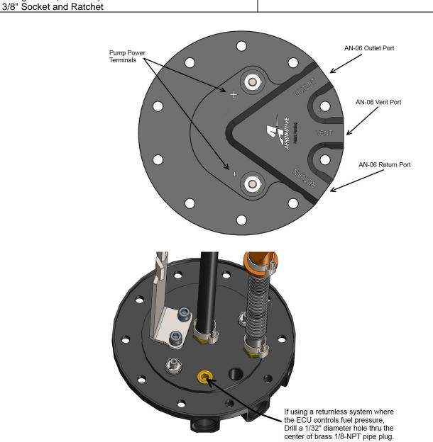
The enclosed Aeromotive fuel pump assembly utilizes an o-ring sealed AN-06 style feed, return and vent ports. These ports seal with o-rings; these ports are **NOT PIPE THREAD** and utilize **NO THREAD SEALANT**.
