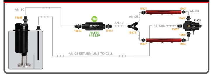
5. If you are running a Carbureted System, connect the fuel filter outlet to a bypass style fuel pressure regulator and/or fuel log as in the following diagrams.
