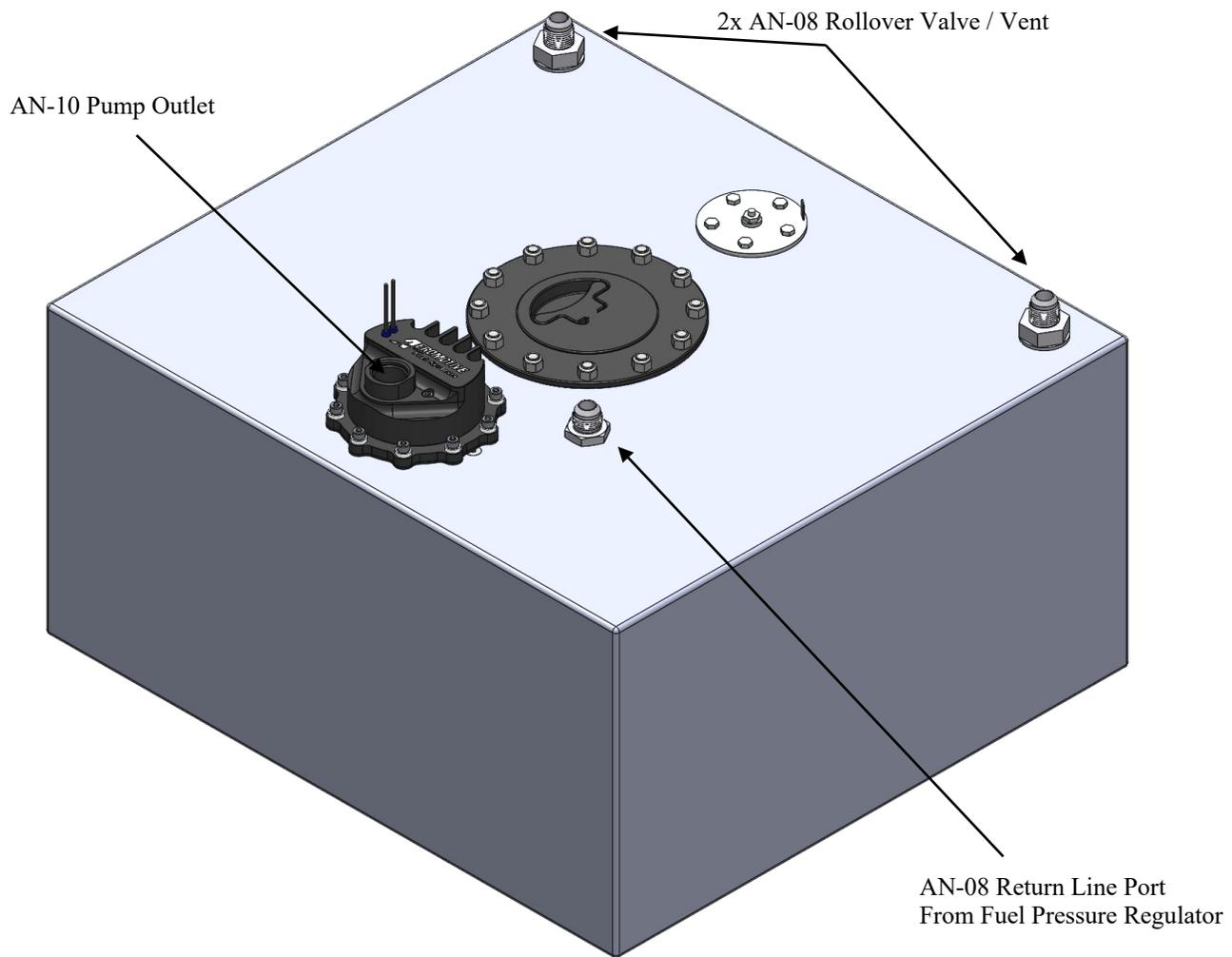
2. Connect AN-08 lines to the tank vent fittings. Tank vent lines must be run outside the vehicle.
