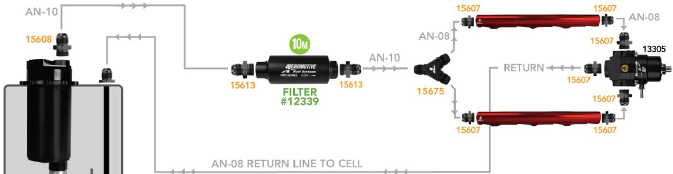
5. If you are running a Carbureted System, connect the fuel filter outlet to a bypass style fuel pressure regulator and/or fuel log as in the following diagrams.
